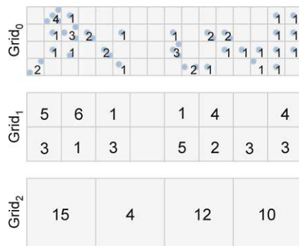
Fig. 2 Mipmap-style computing of coarser-level grids (the number of triangles per cell is highlighted). 2D-projection
