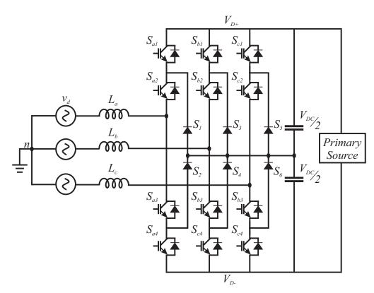
Figure 5. Three-Level NPC Converter Topology.
