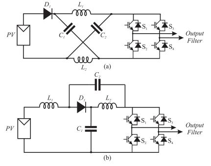
the Z-source and quasi-Z-source single-phase converter schematics, where  $L_1$ ,  $L_2$ ,  $C_1$ , and  $C_2$  constitute the impedance network.
