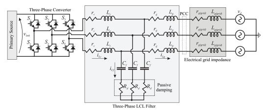
Figure 12. Diagram of a general three-phase grid-connected converter with an LCL filter.
