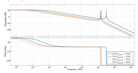
**Figure 13.** Bode diagram of a grid–connected converter with LCL filter under grid impedance variation.
