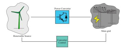
Figure 1. Power Converter Interconnection.
