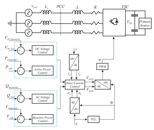
Figure 6. Vector-Controlled VSC Architecture.
