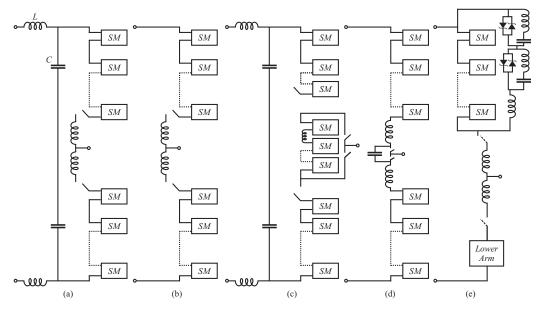
**Figure 8.** Parallel-Connected Topologies: (a) Short Overlap, (b) Extended Overlap, (c) Shared Alternate Arm, (d) Improved Alternate Arm, (e) Augmented Trapezoidal Arm.
