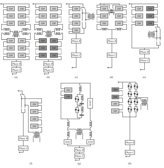
Figure 9. Series-Connected Topologies: (a) Series-Connected, (b) Series-Connected Asymmetrical Hybrid, (c) Series Hybrid Multilevel Converter, (d) Modular Directed Series, (e) Series Bridge Converter, (f) Series Half-Bridge Hybrid Multilevel Converter, (g) Thyristor-Augmented Modular Bridge Converter, (h) METDC.
