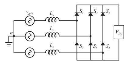
Figure 2. Six-Pulse Converter Topology.
