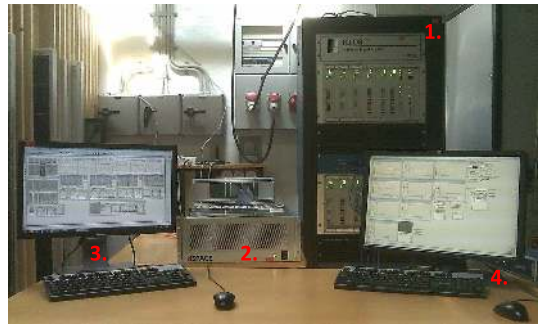
Fig. 2. Photo of the laboratory setup: 1. RTDS, 2. dSPACE, 3. Computer with RSCAD (RTDS simulation control) and 4. Computer with ControlDesk (dSPACE simulation control).
