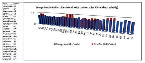
Figure 8 Energy cost of 3 kWp rooftop solar PV in Indian cities (without subsidy).
