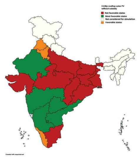
Figure 18 Country Map for 3 kWp rooftop solar PV without subsidy.
