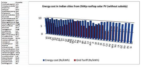
Figure 10 Energy cost of 2 kWp rooftop solar PV in Indian cities (without subsidy).
