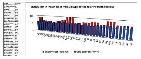
Figure 7 Energy cost of 3 kWp rooftop solar PV in Indian cities (with subsidy).
