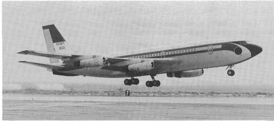
Fig. 1 Boeing-720 controlled impact demonstration (CID) test aircraft.
