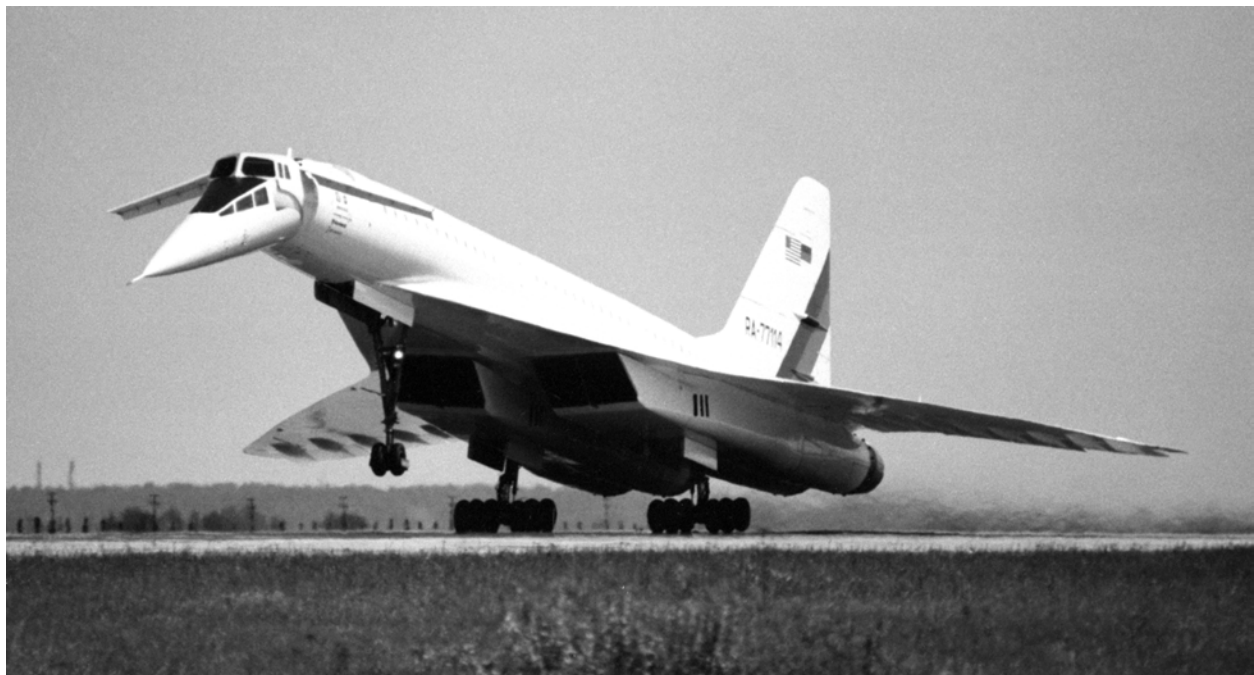
Figure 2. Tu-144LL airplane in the normal landing configuration.
