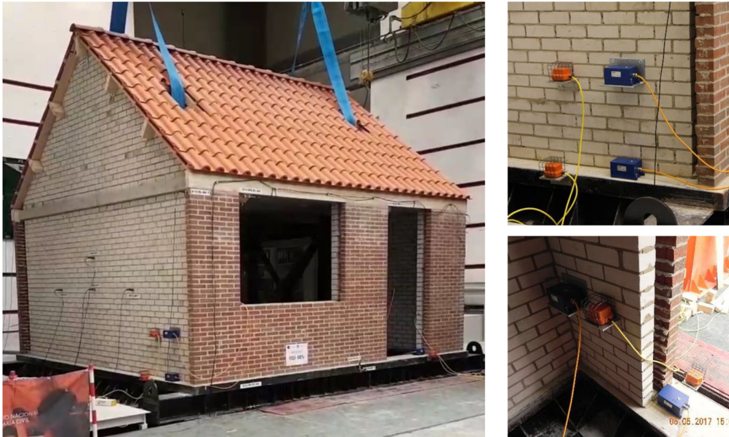
Fig. 16 The specimen house during the first shake table test at the LNEC in Lisbon (LNEC-BUILD1). Six sensors are visible: two installed at a height of 0.45 m on the eastern wall (made of white calcium-silicate bricks), two installed on the eastern wall's foundation base (detail in top right frame) and two on the northern
