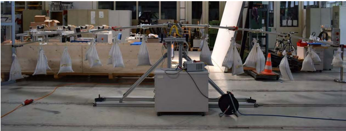
Figure 16. Wings mounted on test-stand for structural airworthiness test - unloaded (above) and loaded (below)
