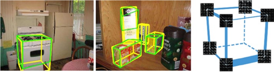
Figure 7-4. Annotated or labeled ground-truth dataset images for scene analysis of cuboids (left and center). The labels are annotated manually into the ground-truth dataset, in yellow (light gray in B&W version) marking the cuboid edges and corners. (right) Ground-truth data contains pre-computed 3D corner HOG descriptor sets, which are matched against live detected cuboid HOG feature sets. Successful matches shown in green (dark gray in B&W version). (Images used by permission © Bryan Russel, Jianxiong Xiao, and Antonio Torralba)
