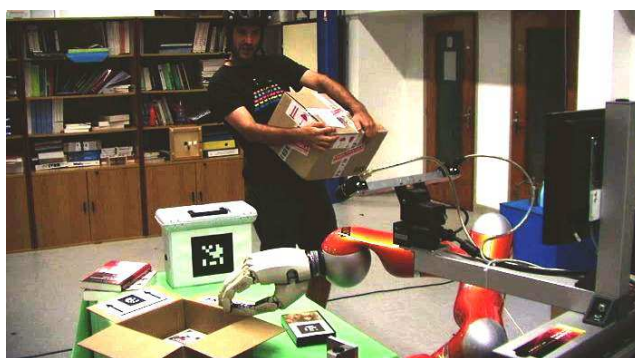
Fig. 1 Interacting with the robot in an everyday setup: the human asks for help in vague terms, the robot takes into account the human’s spatial perspective to refine its understanding of the question.
