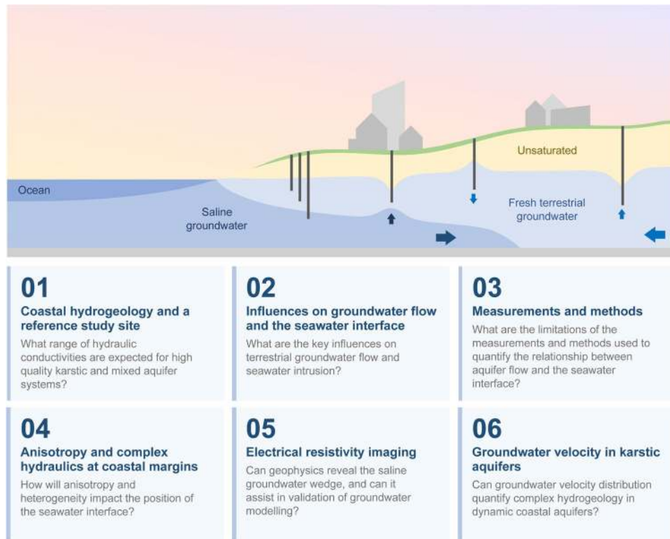
Figure 1. Schematic of a shallow coastal groundwater water system in an urban setting and our research outline. The multidisciplinary research is partitioned into six connected parts spanning geology, method of acquisition and processing of well data, numerical groundwater modelling and geophysical methods. An example of the type of questions addressed in each part is provided.
