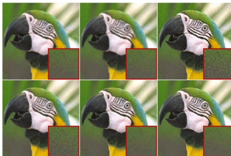
Fig. 8 Comparison of SR results of parrot image with noise level \sigma_v = 5 with magnification factor 2. Top row : input image, bi-cubic, and the method in [20]. Bottom row : the method in [15], the method in [13], and the proposed method
