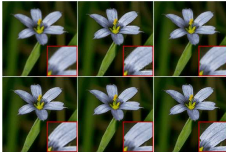
Fig. 4 Comparison of SR results of blueeye image with magnification factor 2. Top row: bi-cubic, the method in [20], and the method in [15]. Bottom row: the method in [13], the proposed method, and the ground truth image
