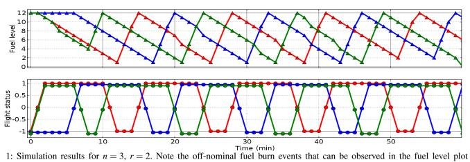
1: Simulation results for n = 3, r = 2. Note the off-nominal fuel burn events that can be observed in the fuel level plot (these are places where the graph has a slope of -2).
