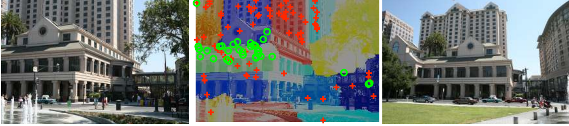
Figure 4. RANSAC can be significantly sped up if modified to take advantage of additional grouping information between features, e.g., as provided by image segmentation. Left and Right: two images for which we seek epipolar geometry. Middle: inliers (green) and outliers (red) overlaid on the image segments: notice the clear correlation between segmentation and inlier/outlier classification.
