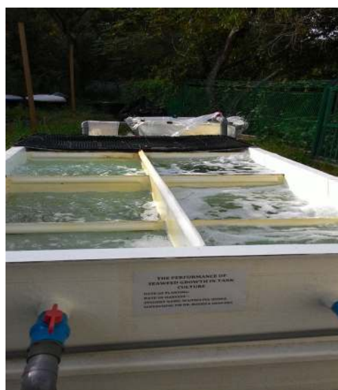
Fig. 1 The customized tank used to culture the seaweed
