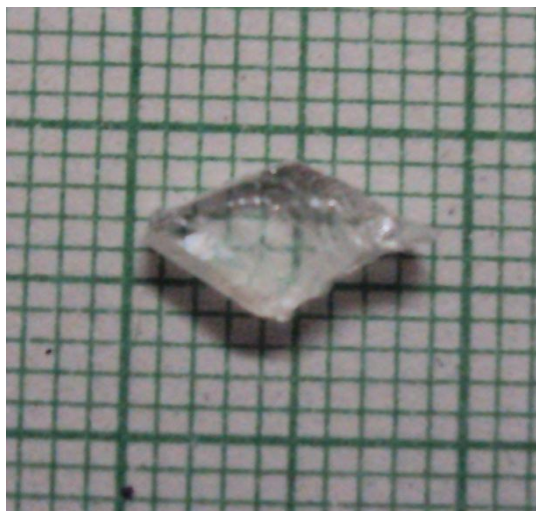
Fig. 1 Photograph of grown single TPM NLO single crystal
