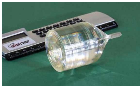
FIG. 5. High quality stoichiometric \text{LiNbO}_3 crystal grown by the HTTSSG method.
