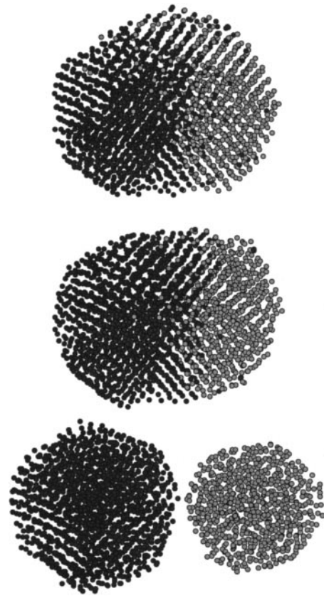
FIG. 36. Successive cluster morphologies during the coalescence of a gold 767-atom liquid cluster with another gold 1505-atom solid cluster. The figures represent three stages of the coalescence process after 0, 1, and 10 ns, i.e., times much longer than those studied by Zhu and Averback (1996).
