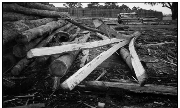
Figure 2. A near-full-length log splitting due to the release of growth stresses following the crosscut ( Eucalyptus spp. )
