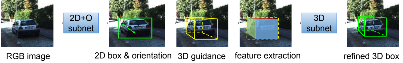
Figure 5. Overview of the proposed 3D object detection paradigm. A CNN based model (2D+O subnet) is used to obtain a 2D bounding box and observation orientation of the object. The guidance is then generated by our proposed algorithm using the obtained 2D box and orientation with the projection matrix. And features extracted from visible surfaces as well as the 2D bounding box of the projected guidance are utilized by the refinement model (3D subnet). Instead of direct regression, the refinement model adopts classification formulation with the quality-aware loss for a more accurate result.
