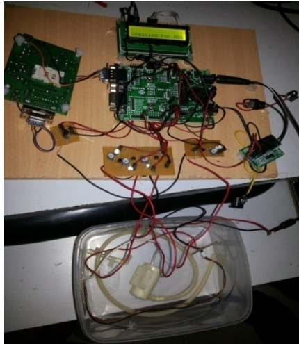
Fig.1: GSM based automatic irrigation control system by using an android mobile
