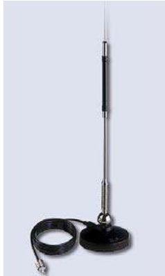
Fig. 6: Used \lambda/4 monopole receive antenna
