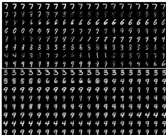
Figure 4: Successive samples generated by Markov chain associated with the trained DAEs according to the plain sampling scheme (left) and walkback sampling scheme (right). There are less “spurious” samples with the walkback algorithm.
