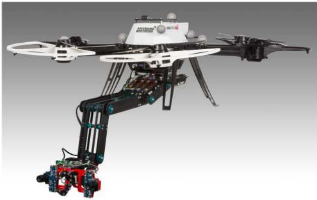
Fig. 1 An aerial robotic worker
