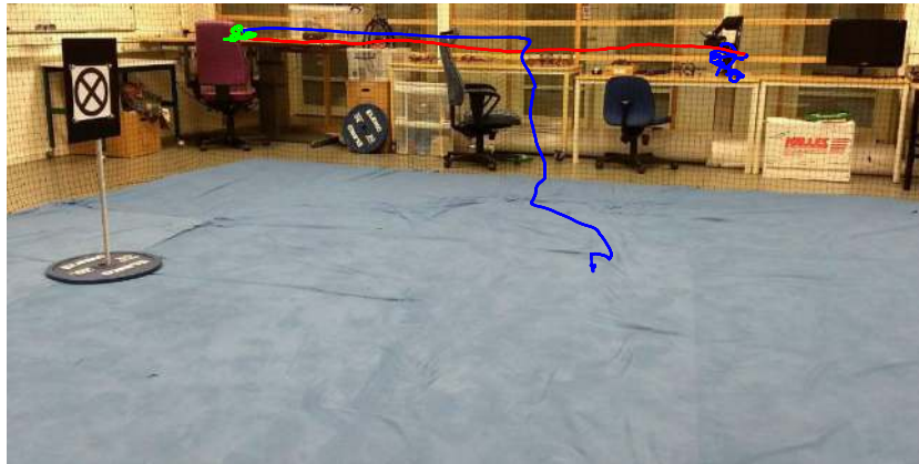
Fig. 9 MAV actual trajectory derived from the experimental trials of the stereo-based guidance. Case 1: relative distance with the target 25 cm. The developed guidance system contributes to the task with the red and green part of the overall trajectory. The red part is followed after the extraction of the centroid, while in the green part the
