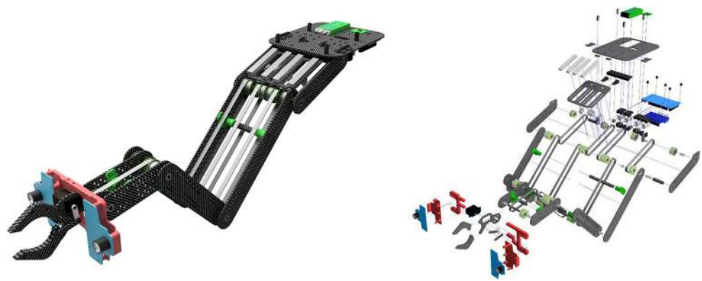
Fig. 2 Left - CAD design of the CARMA manipulator. Right - CARMA parts explosion view (Video Link at [14])
