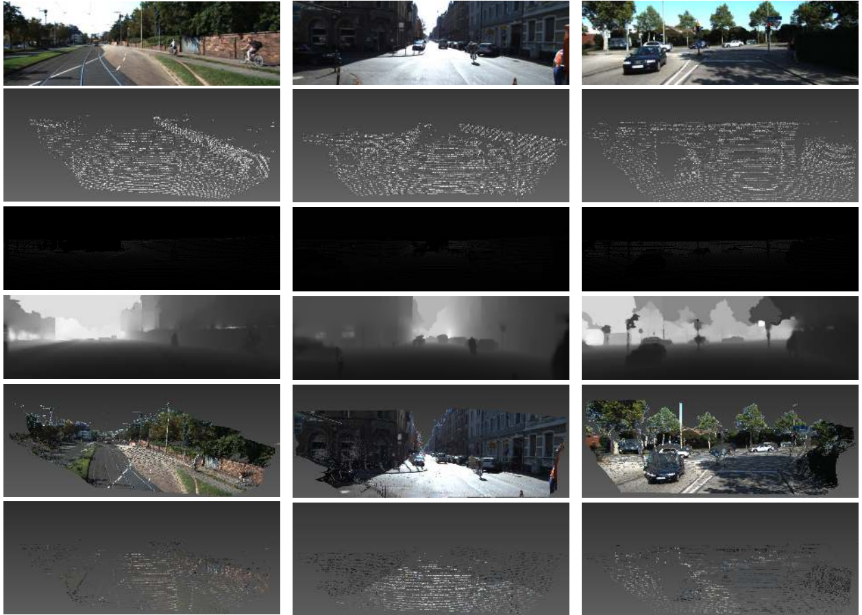
Figure 3. Results of the guided depth upsampling performed on a Velodyne 64E Lidar dataset. The first two rows, respectively, are high-resolution color images and sparse 3D lidar points. The third row contains low-resolution maps obtained by registering 3D points to the images. The fourth row presents upsampled depth maps, and the fifth shows the rendered dense 3D point clouds obtained from our upsampling results (sky regions are removed). For comparison, the sparse rendered 3D point clouds are also provided in the last row.
