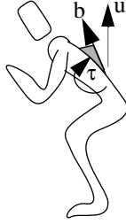
Fig. 4. The hand of God (HOG). The HOG operates by applying an external torque vector \tau to ensure that the up-vector b , fixed to the torso, never deviates significantly from its ideal direction given by u .
