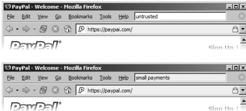
FIGURE 13-14. The petname toolbar, shown in untrusted (top) and trusted (bottom) states, supports user-assigned site names
