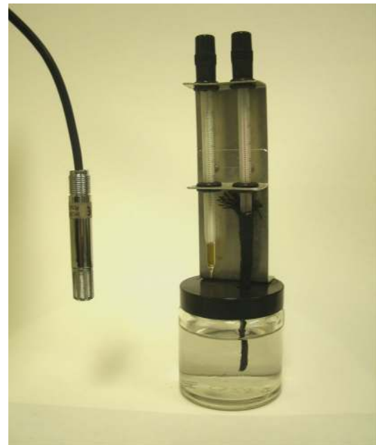
Fig. 2 Water vapour (humidity) sensors may be relatively inexpensive capacitance hygrometers ( left ) or a basic psychrometer ( right ).
