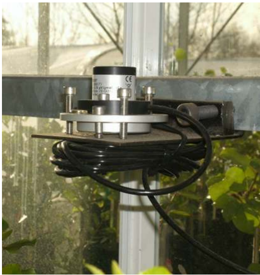
Fig. 1 A quantum sensor on a leveling platform mounted at the top of the canopy for measuring photosynthetically active radiation (PAR). Radiation sensors should be chosen for the specific purpose required. Positioning should be carefully considered to avoid shading or noise from reflective surfaces.
