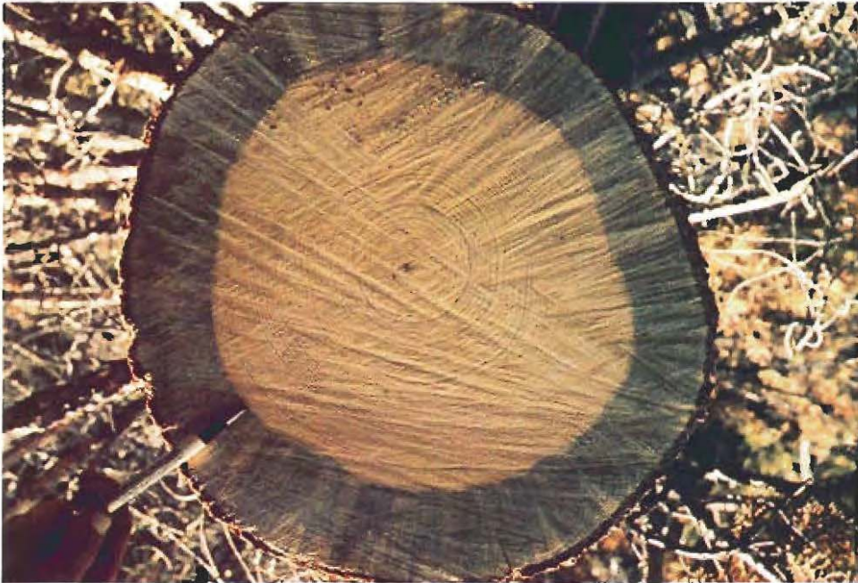
Figure 8.--Blue-staining fungi, carried into the bark by the beetles, discolor the sapwood. A. Well-developed blue stain usually is uniformly distributed throughout the sapwood. B. Poorly developed blue stain usually is unevenly distributed in the sapwood.
