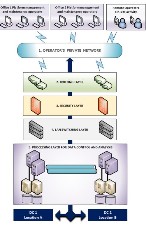
Figure 1. Computing core group architecture.
