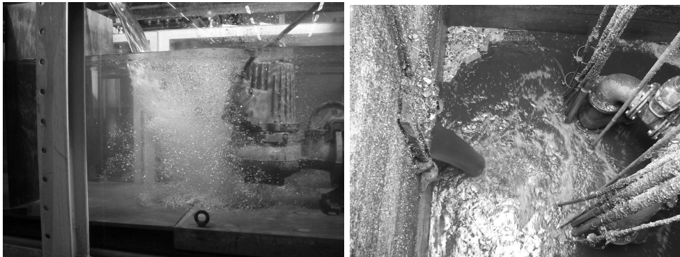
Figure 1: Air entraining plunging jets in the lab [3] and the field
