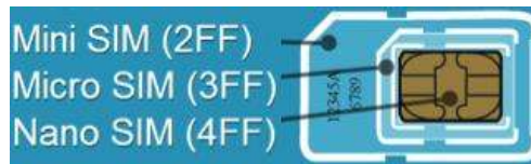
Figure 2: SIM Card Size Formats [Orm09]
