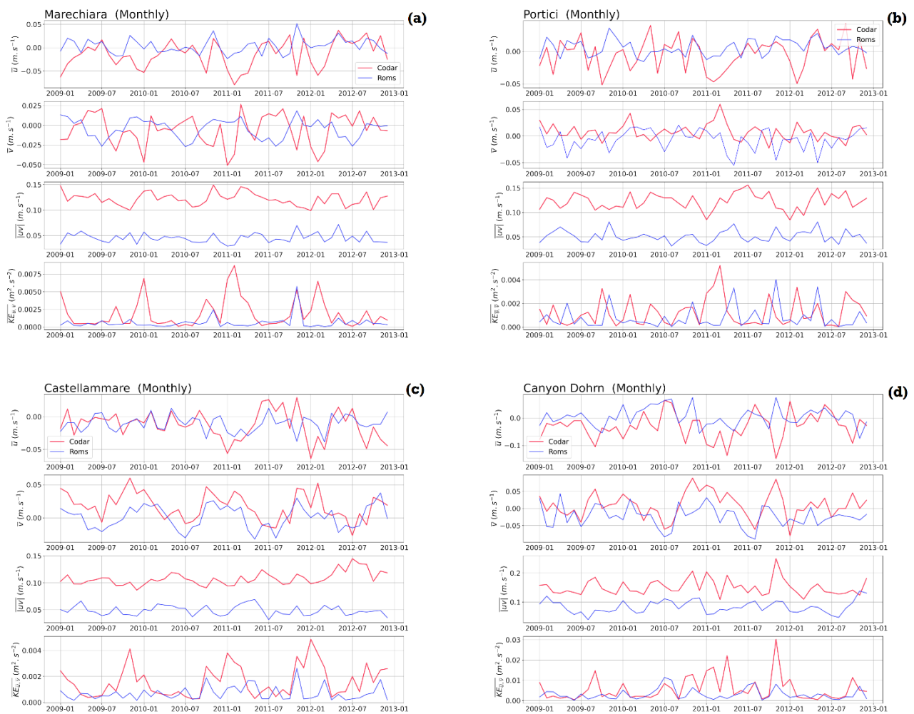
Figure 9. Time series of the monthly averaged velocities (components u , v , and module) and their associated kinetic energy at the four specific areas: (a) Marechiara, (b) Portici, (c) Castellammare and (d) Canyon Dohrn. Red: HFR observations; blue: GNAM model.
