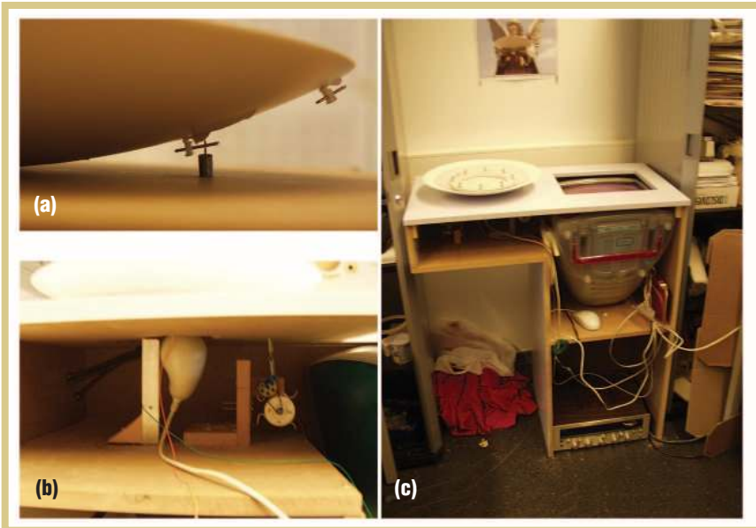
Figure 7. A high-tech prototype's technical construction. (a) The bowl is connected with a spring to an electromotor, (b) a camera with fisheye lens is positioned pointing upwards below the bowl, and (c) a PC connects all elements.
