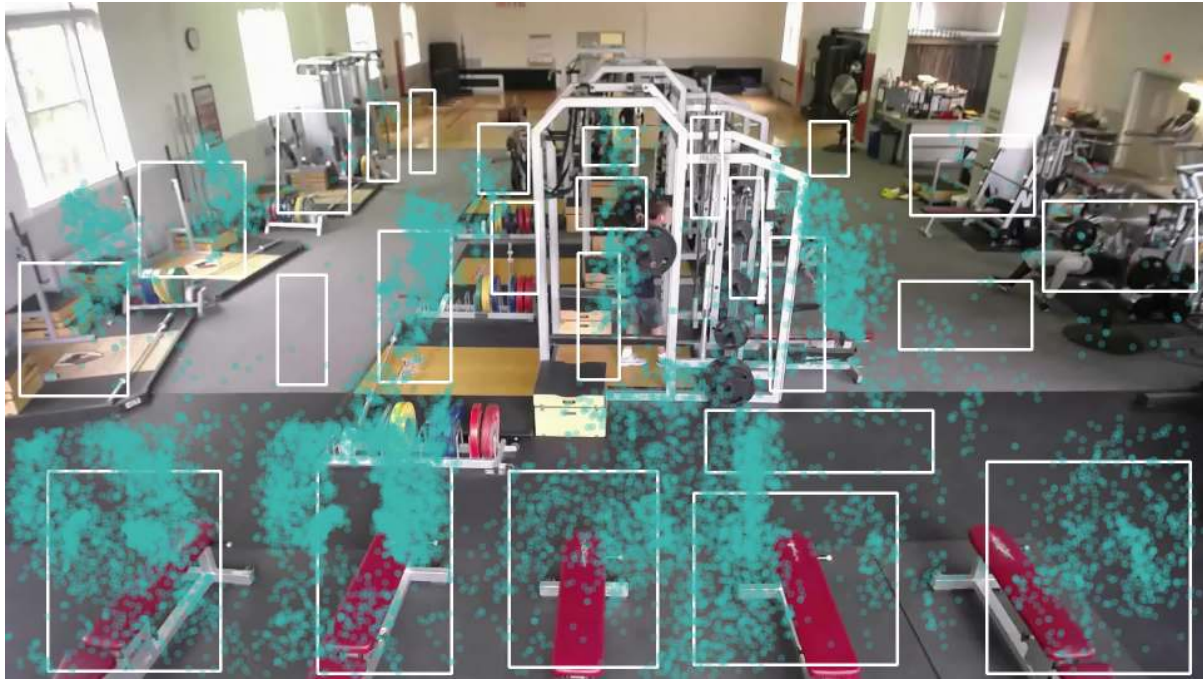
Fig. 7. An image of the gym with a distribution of all the exercise motions observed across all videos. The white boxes are the manually-drawn boxes to aid in clustering.
