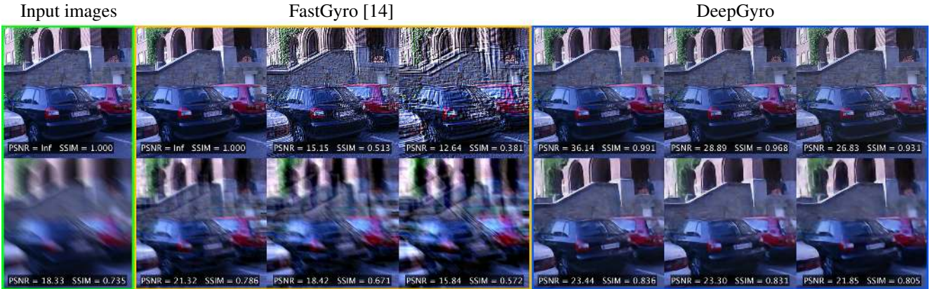
Figure 7. The effects of blur estimation errors on the FastGyro [14] (orange) and DeepGyro (blue). Showing the results when the input is sharp (top row) and when it is blurred (bottom row). The error of the blur is gradually increased \epsilon = k * [5, 3] pixels, where k = 0, 2, 4 .
