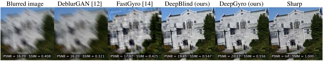
Figure 5. Deblurring results on an image with synthetic linear blur, length 60 pixels. The blur passed to the non-blind methods – FastGyro and DeepGyro – is biased, \epsilon = [5, 3] pixels is added to the blur vector in the x and y directions, respectively.
