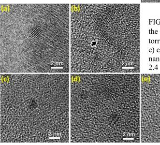
FIG. 3. Selected HRTEM images of Pt NPs on the  $\gamma$ -Al<sub>2</sub>O<sub>3</sub> support in the ETEM column of 1torr H<sub>2</sub>: (a) 2 nm particle at 385 °C, and then (be) cooled down to RT; the crystalline nanoparticle sizes are (b) 1.2 nm, (c) 1.4 nm, (d) 2.4 nm and (e) 2.6 nm, respectively. Pt NPs
