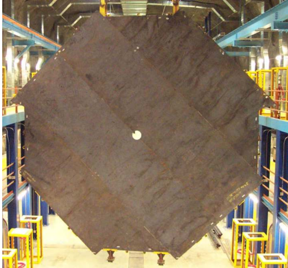
Figure 3.1: A Far detector steel plane being hoisted inside the Far detector cavern. The plane is 8 meters wide.
