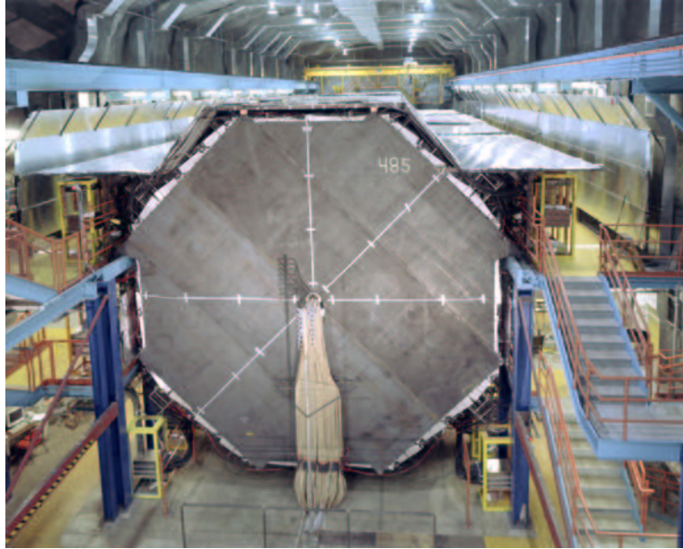
Figure 3.9: The Far detector as it was after completion in July, 2003. Scintillator planes line the top and sides of the detector forming a veto-shield used to suppress downward going cosmic rays [39].
