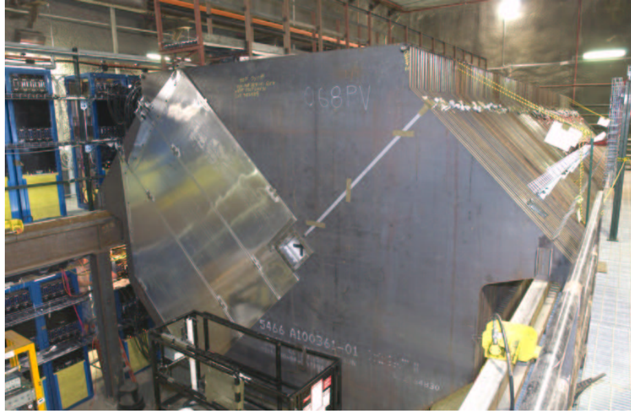
Figure 3.10: The Near detector on July 9, 2004. At the time the photo was taken the detector was still being installed. The leading plane is partially instrumented and in the Hadron Calorimeter section of the detector [39].
