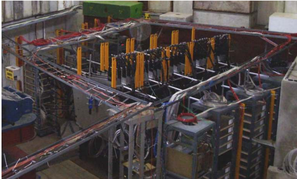
Figure 3.11: The CalDet in T7 beamline of the CERN East Hall during 2002. Phototubes reside inside the metallic mux-boxes located in the racks alongside the detector.
