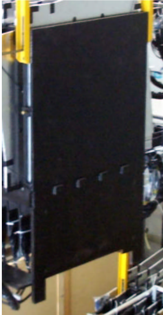
Figure 3.3: A CalDet steel plane. The plane is a 1\text{ m} \times 1\text{ m} square and rests atop a \sim 80\text{ cm} high base.
