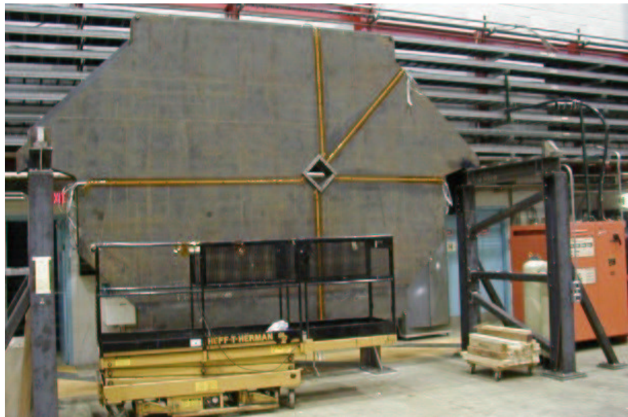
Figure 3.2: A Near detector steel plane. The plane is 6.2 m wide and 3.8 m across.
