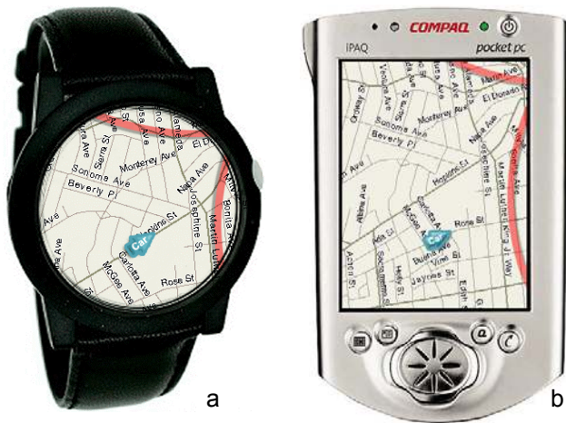
Figure 6: (a) On a circular display, arcs representing the same distance have the same length. (b) On a rectangular display, that is not always the case, because arcs in corners may be cropped.
