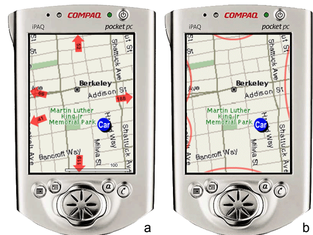
Figure 8: (a) The Arrow interface and (b) the Halo interface, both showing the same map. Which of the 5 off-screen restaurants is “closest” to the car?
