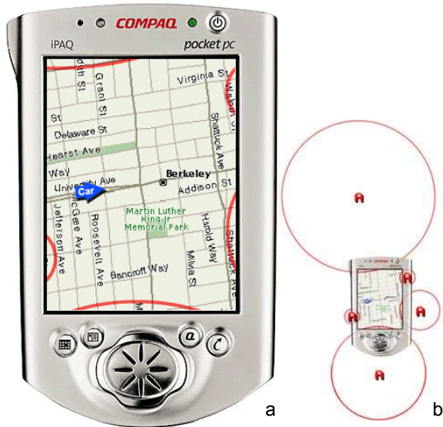
Figure 2: (a) Enhancing the map from Figure 1 with Halo shows where in off-screen space the five restaurants are located. (b) How it works: each off-screen location is located in the center of a ring that reaches into the display window.
