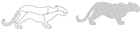
Figure 7. Left: A subpixel medial axis, with branch points shown as empty circles and end points as filled circles. Compare with the results in Fig. 5. Right: The reconstruction as the envelope of the maximal inscribed disks (grey) of the medial axis, overlaid on the original shape.
