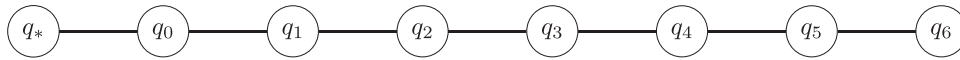
Fig. 1 Connectivity graph for qubits in our model. Each circle represents a qubit. Qubits connected by a solid line can have the Heisenberg interaction applied between them. The qubit q_* can be prepared in the state |0\rangle or |+\rangle
