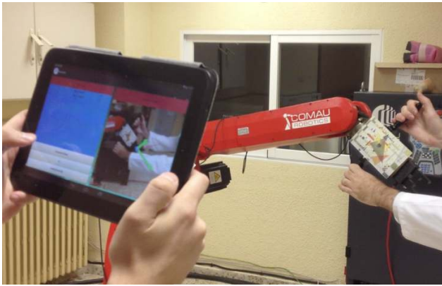
Fig. 10. Augmented reality example: showing force vector
