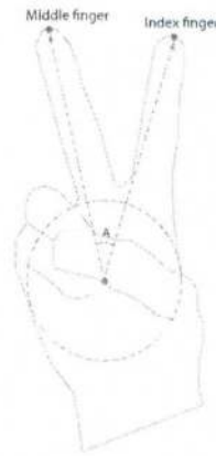
Figure 7. Recognition Example. In the first layer, the system determines that the number of fingers in this gesture is two. Then in the second layer, the finger names of “index finger” and “middle finger” are found. The classifier in the third layer calculates the angle of two finger vectors are within a range of 30 degree to 60 degree. Thus the gesture is recognized as “Victory” in the Popular Gesture scenario, while in the Numbers scenario it is recognized as the number “Two” through a similar process.
