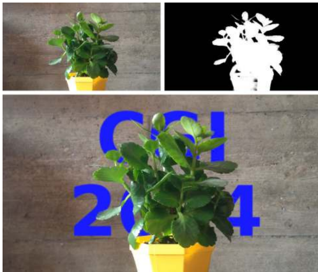
Fig. 9 An application of our computed alpha matte: for the reference image ( top left ) an alpha matte is generated for the foreground ( top right ). The object is inserted into the scene and blended with the foreground ( bottom )
