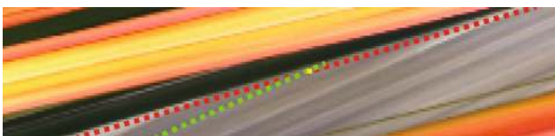
Fig. 5 The accumulated score of the red disparity hypothesis is larger than the one of the green one because we find more pixels with non-zero scores along the red line . On the other hand, the green hypothesis has fewer but higher non-zero scores. Our normalization gives preference to the correct hypothesis in green
