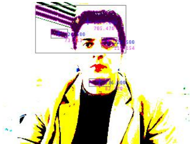
Fig 1. Numerous blobs were extracted from the source image by using OpenCV Blob Extraction library.
