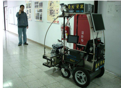
(a) A person interacts with the NTU PAL1 robot via hand posture.
