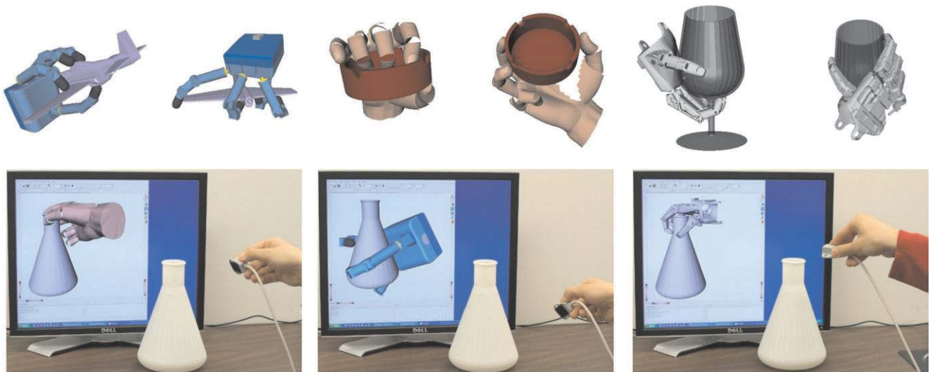
Fig. 13. Examples of interactive grasping tasks executed in simulated environments. Bottom row images also show the user providing the approach direction via a magnetic tracker. All of the presented grasps have form-closure.
