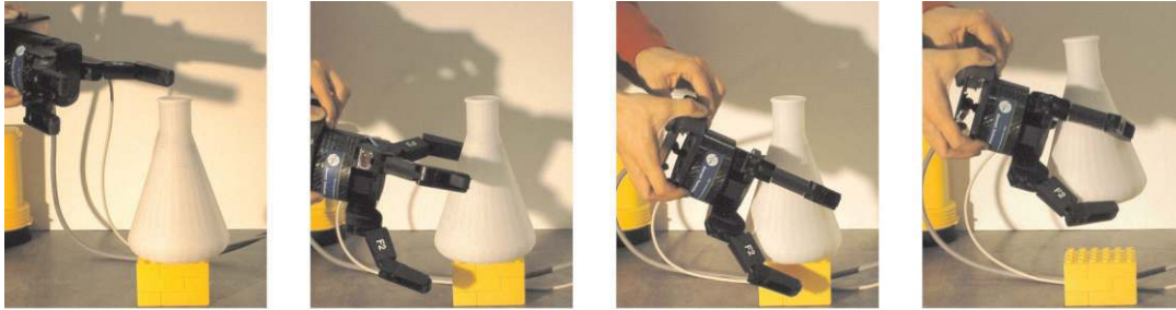
Fig. 11. Example of a complete grasping task: initial approach, finger pre-shaping using grasp planning result, continued approach and final grasp execution.
