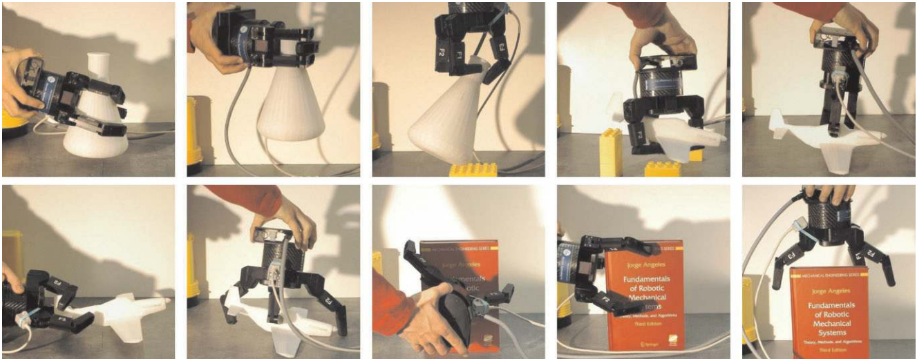
Fig. 12. Examples of interactive grasping tasks; each image shows the grasp found for a different approach direction or target object. In all cases the object was successfully grasped and lifted off the table.
