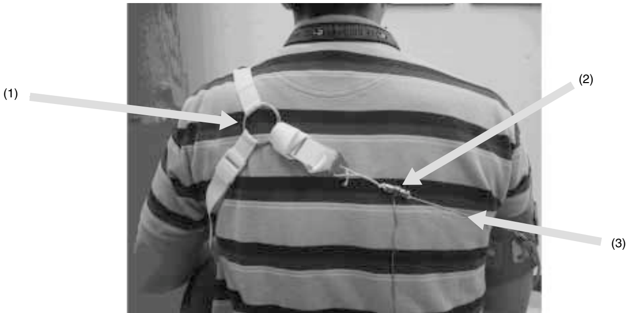
Figure 1. Back view of cable orthosis showing figure-of-eight harness (1), in-line load cell (2), and cable (3).
