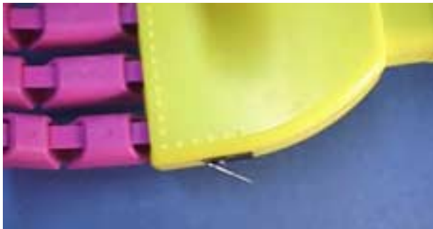
Fig.5 The micro-switch sensor on the bottom side of the Hand Part
