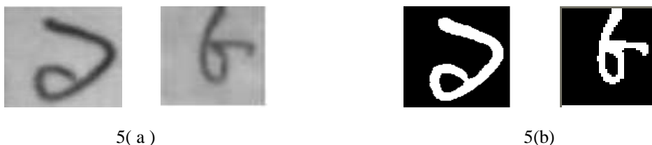
Fig-5: (a) preprocessed image, (b) resultant image after Region Probability Estimation and Region Classification
